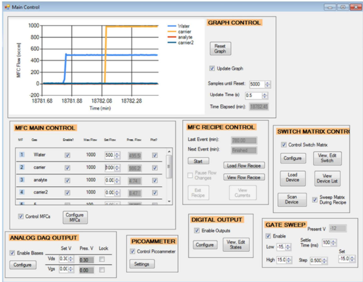
Figure 5.2: Front panel of the program used to control the vapor sensor setup. A flow rate recipe can be loaded and monitored. Simultaneously, a switching matrix is used to cycle through a desired set of up to 100 devices. The bias voltage and gate voltage – static or sweeping – that are applied to the devices can also be preset. The program can run for hours or overnight without the need for user input.
